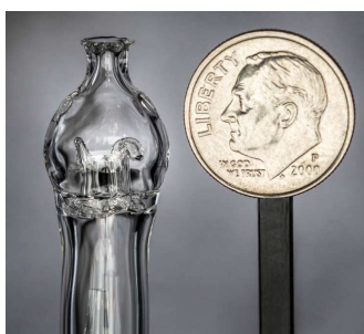
Fig. 1. The quartz supercritical-pressure jet stirred reactor [17]
