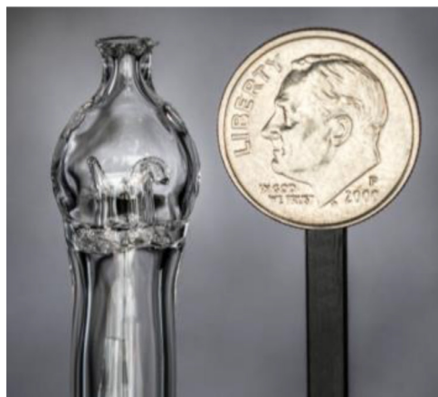
Fig. 1. The quartz supercritical-pressure jet stirred reactor [17].
